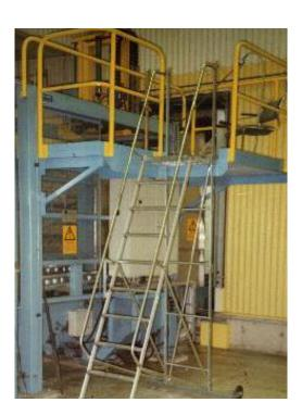
The AutoStripper® Unit is specifically designed for dewiring of market pulp bale units in pulper charging lines. AutoStripper Unit mainly consists of at cutting unit, a pair of wire holding arms, a wire winder and a belt conveyor to bring the coil to the scrap bin. The closed design assures that no wires with spring back can cause accidents.
