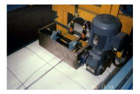
The cutting unit operates from the top. To avoid contamination of the pulp no hydraulics are used for cutting.
