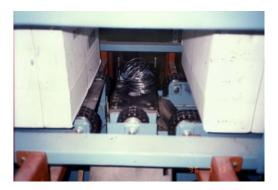
The scrap coil before being conveyed to the bin.
