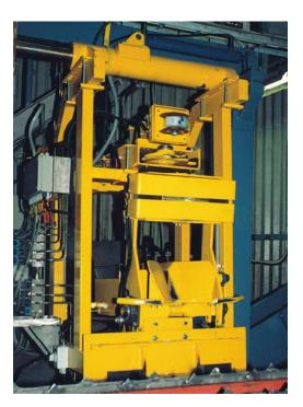
The AutoStripper® Unit Compact has been developed for low and medium capacity mills, where cost efficiency and space saving are key features.
