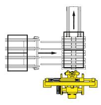
In an angle, where the bale units are loaded to the system across the conveying direction.
