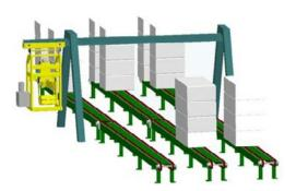
Traveling along an overhead beam across several loading conveyors.
