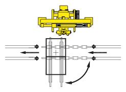
In-line, where the bale units are loaded to the system along the conveying direction.
